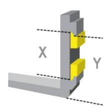
Respecting the carriage dimensional tolerances, hook type forks can have a wide range of blade lengths and section sizes.
